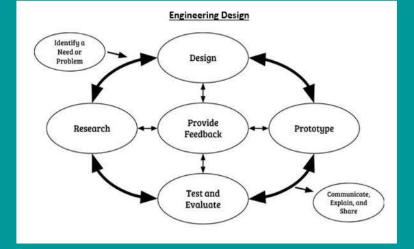
A prototype is constructed based on the design model(s) and used to test the proposed solution. A prototype can be a physical, computer, mathematical, or conceptual instantiation of the model that can be manipulated and tested.
