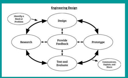
Identify a need or a problem. To begin engineering design, a need or problem must be identified that an attempt can be made to solve, improve and/or fix. This typically includes articulation of criteria and constraints that will define a successful solution.
