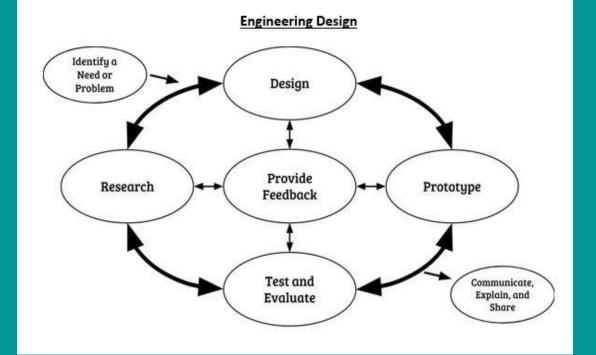
The feasibility and efficiency of the prototype must be tested and evaluated relative to the problem criteria and constraints.
