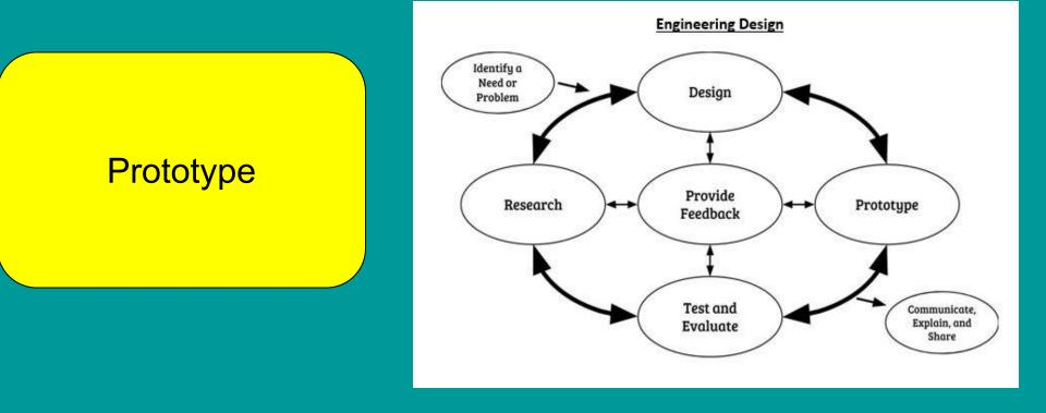
A prototype is constructed based on the design model(s) and used to test the proposed solution. A prototype can be a physical, computer, mathematical, or conceptual instantiation of the model that can be manipulated and tested.
