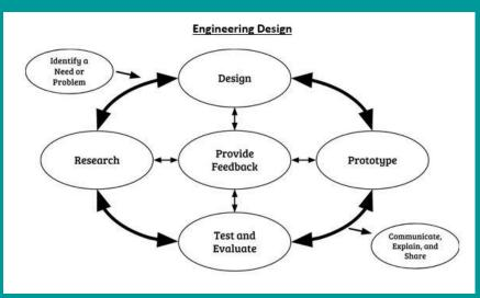
Identify a need or a problem. To begin engineering design, a need or problem must be identified that an attempt can be made to solve, improve and/or fix. This typically includes articulation of criteria and constraints that will define a successful solution.
